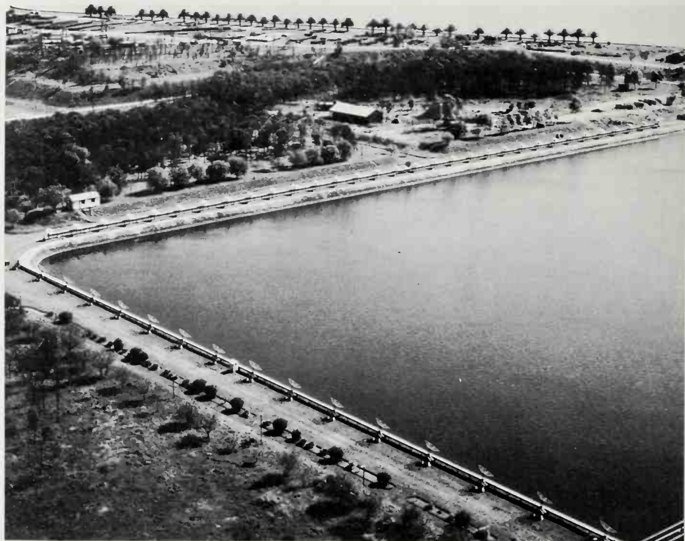
The two grating interferometer radio telescopes at Potts Hill, Sydney, Australia. These can be used together to make a rotational synthesis instrument.
