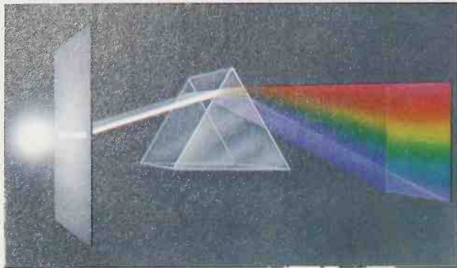
Fig. 3-2 When white light is passed through a prism it is split into many colours known as a spectrum. This rainbow-like effect was first studied in 1665 and 1666 by Sir Isaac Newton. Light of different wavelengths is deviated by varying amounts as it passes through the glass prism, red light being deviated least. This simple experiment shows how white light is a mixture of all colours between red and violet.
