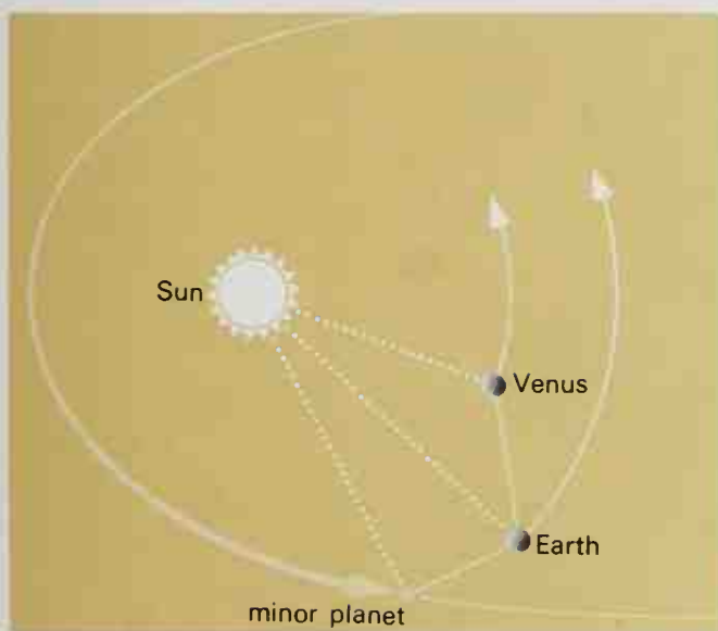
Fig. 2-11 above: Determination of the astronomical unit. Determination of the Earth-Venus or Earth-planetoid distance by radar, allows the Earth-Sun distance (which cannot be directly measured) to be calculated by simple trigonometry, as all the angles in the triangle are already known.
