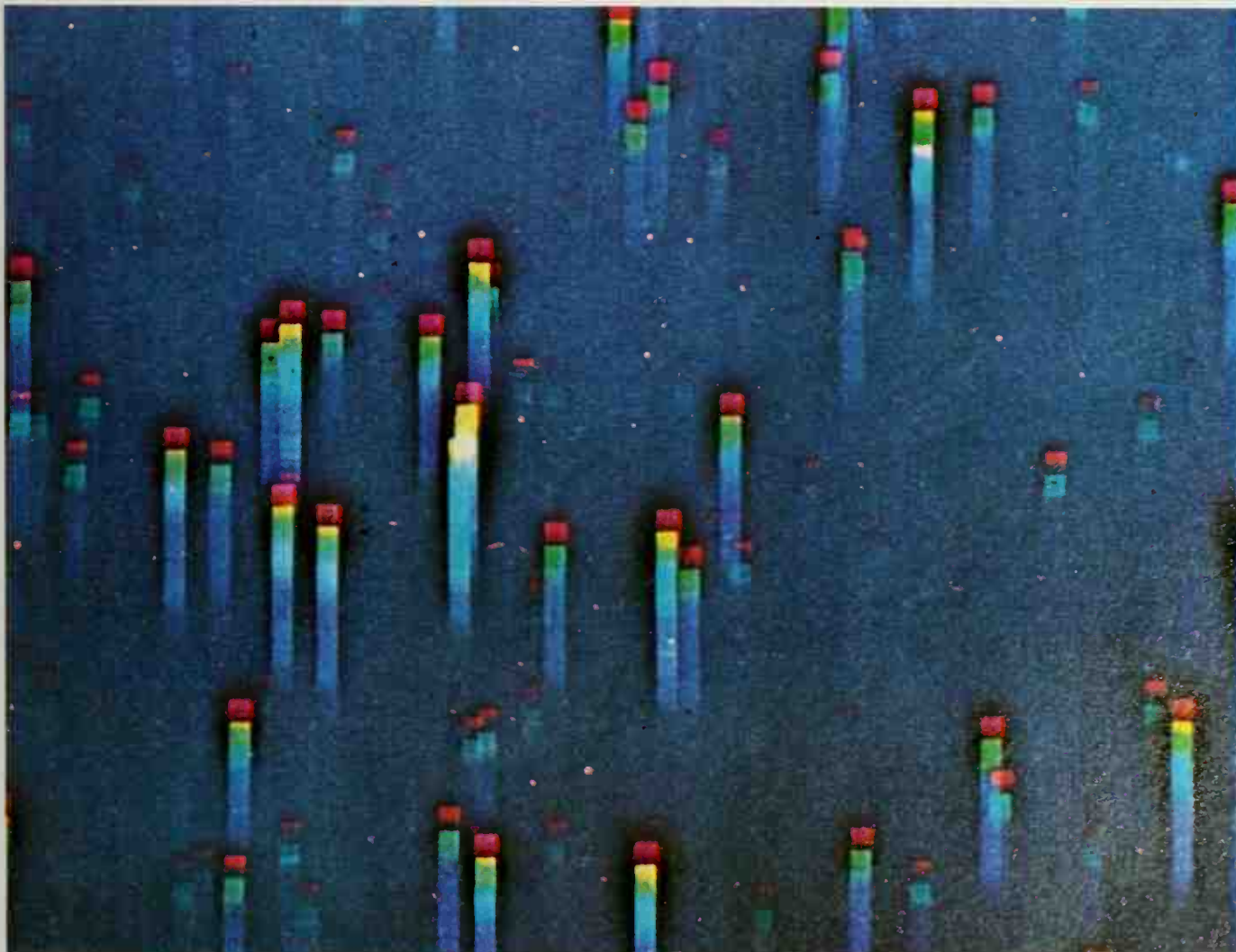
A low dispersion spectrum of the Hyades star cluster obtained with a device known as an objective prism: a large prism placed at the front aperture of the telescope thus enabling the spectrum of each star to be obtained simultaneously.
